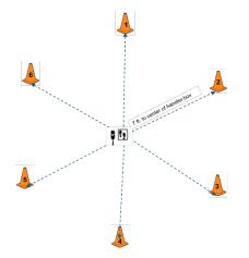
Cones are positioned 7ft from the centre of the handler box.
